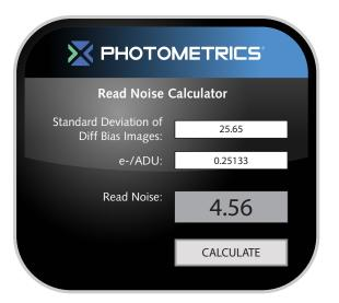
Read noise is the amount of noise generated by electronics as the charge present in the pixels is transferred to the camera. It is a combination of all the noise generated by system components which convert the charge of each CCD pixel into a signal for conversion into a digital unit (ADU or grey-scale value). Since read noise is added to each pixel as it is read out, it is applied uniformly across the CCD as the data is read out.
